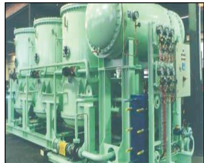
Multi Stage Flash (MSF) Evaporators
